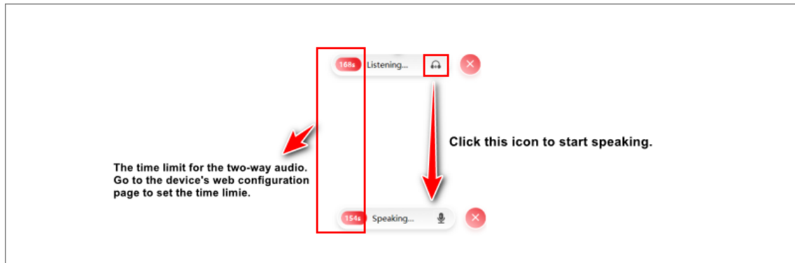
Figure 4-9 Two-Way Audio with Half-Duplex Sounder
